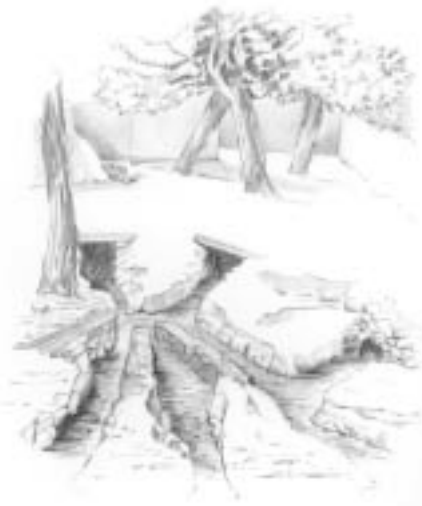
Figure 5 A Water Divider in Mahan. Two granite blocks were imported to Mahan to build a maqsam which subdivided the water emerging from two qanats into three major streams ( shahjub ) of equal flow. At some past time, one of the granite blocks was dislodged by a flash flood. Because of disagreement about its precise location prior to the flood, it was never repositioned. The owners of the major stream on the right clearly gained water because of the new position of the divider after the flood. The owners of the central stream lost water. Note that a third qanat enters the stream on the right below the maqsam . (Illustration by Ann Coffin Delano)
